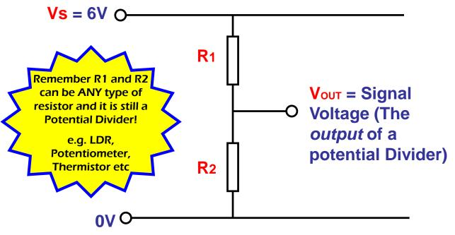
Each resistor *reduces the voltage* a bit so the *supply voltage gets "divided"* between the 2 resistors depending on their value.
